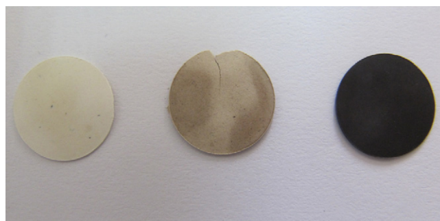
Fig. 8. Photography of three Avicel pellets: (A) raw cellulose fibres; (B) amine-functionalised fibres after interaction with the \text{AgNO}_3 solution at room temperature for 30 min; (C) amine-functionalised fibres after interaction with a \text{NaAuCl}_4 solution at 70^\circ\text{C} for 30 min.
